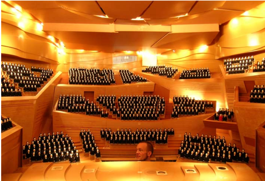
Figure 1: The 1:10 scale model of the new Danish Radio concert Hall. View from the organ towards the seat sections in front of the stage. The head of the author's son has been used to indicate the dimensions.
