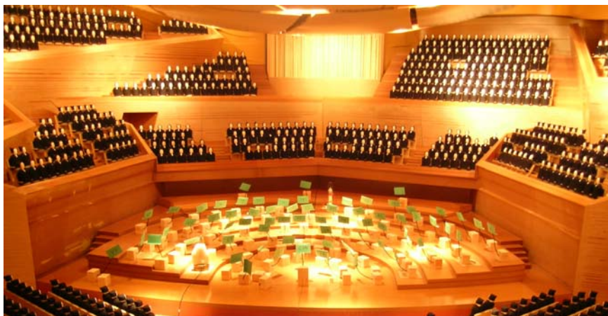
Figure 2: View towards the furnished stage in the 1:10 scale model of the new Danish Radio concert hall.
