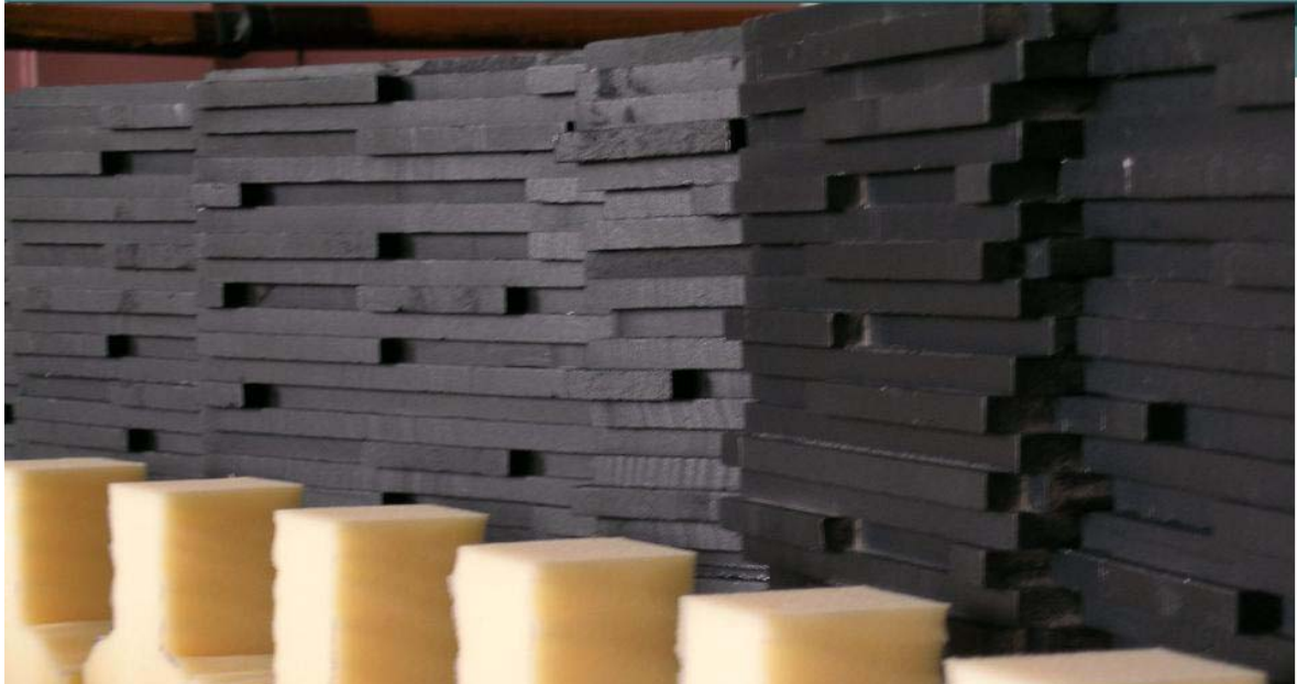
Figure 5: detail of 1:5 scale model brick wall for the main auditorium in the new Royal Drama Theatre in Copenhagen The white cubes in front are "heads" of model audience.
